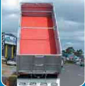
RED HOT LINER FOR HOT ASPHALT TO 205°C
