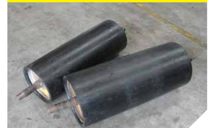
Conveyor Belt Pulleys
