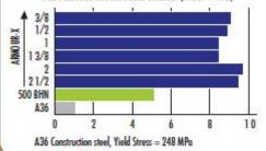
The superior wearability of ARMOUR.X is achieved through new 21st century alloy steel technology. The result is a Formable, Weldable wear plate in the 450 BHN range that offers wear resistance almost twice that of conventional 500 BHN grades.
