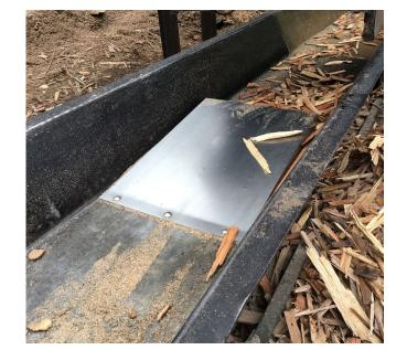
As material is conveyed over the VIBRA-SEP face, tramp metal is captured to the trailing edge thereby removing tramp from the product flow. Removal of the retained tramp is done by simply sliding the captured contaminates off the VIBRA-SEP.
