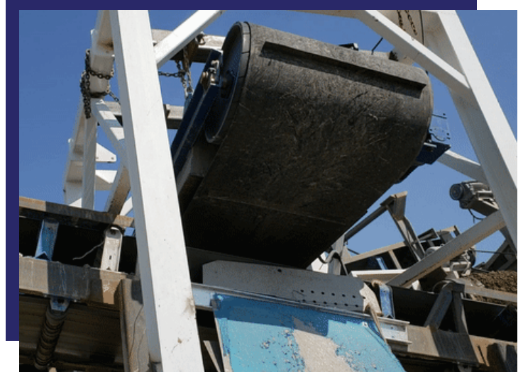
SELF CLEANING ELECTROMAGNETIC SEPARATOR DISCHARGING TRAMP METAL TO A CHUTE
