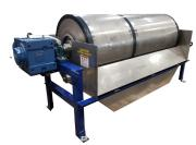
Wet drum separators are commonly used in slurry applications for mining operations with heavy media circuits and iron ore concentration.
