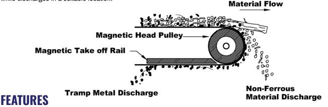
It is critical to select the correct magnetic pulley for your operation; standard applications typically require IMT deep reach ceramic magnets while IMT high intensity neo rare earth magnets are used in more aggressive applications.
