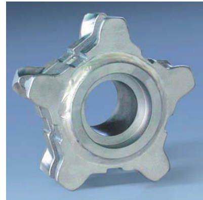
Figure 48: HEKO chain wheel type GTE, pocket teeth, one-piece, welded steel fabrication
