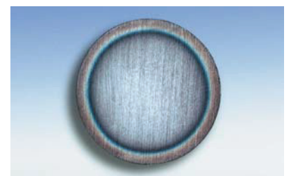
Figure 4: Cross section through the wire diameter of a case hardened chain link
