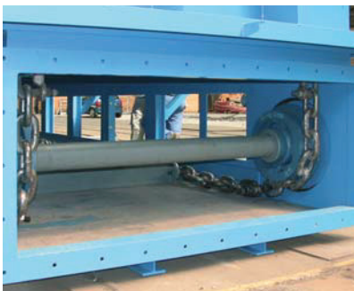
Figure 65: drive unit, tensioning unit diversion for SCC, using HEKO compo- nents
