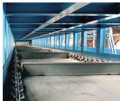
Figure 62: HEKO chains, scraper attachments in lower trough of SCC
